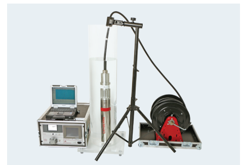
Sealed HPGe in water tank (25 m cable)
